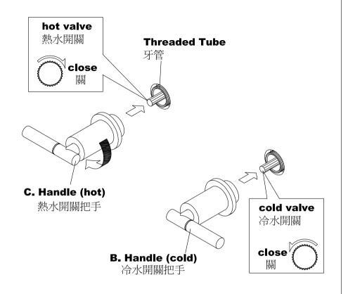
\* Turn hot valve clockwise and cold valve counterclockwise to closed position before install Handle Assembly. Keep both hot and cold Handle Assembly lever faces horizontal, then press each Handle Assembly onto valve spindle and securely hand tighten the Handle Assembly against finished wall.
