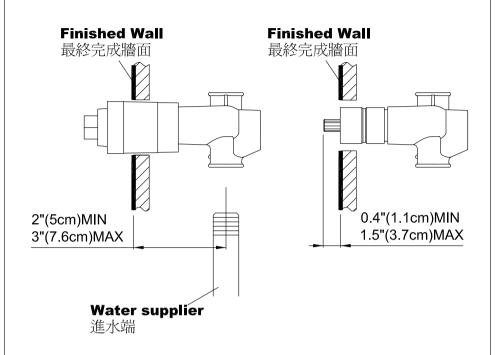
\* Connect hot and cold supplies pipes to the valve body, so they are between 2"(5cm) minmum and 3"(7.6cm) maximum from the finished wall; or keep the distance be 0.4" (1.1cm) to 1.5" (3.7cm) between top of cartridge and **Finished Wall** for necessary conditions.
