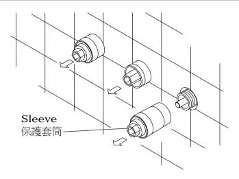
$^{\star}$  Remove the Sleeves after complete the finished wall for installing the Handle and Spout.
