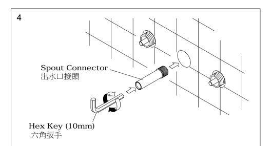
\* Apply pipe compound or thread sealant tape to the thread of Spout Connector, screw the Spout Connector to the Valve Body with Hex Key(10.0mm), and then cover with Plate.
