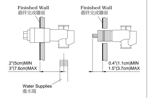
\* Connect hot and cold supply pipes to the Valve Body, and keep the distance between 2" (5cm) minimum and 3" (7.6cm) maximum from the Finished Wall to the center of Valve Body; or keep the distance be 0.4 " (1.1cm) to 1.5" (3.7cm) between top of cartridge and Finished Wall for necessary conditions.
