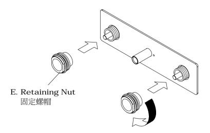
\* Fix the Plate against wall with Retaining Nut. Insert the Spout Connector into Spout to make Spout be flush with Plate; tighten the Set Screws underneath Spout with Hex Key(2.0mm).
