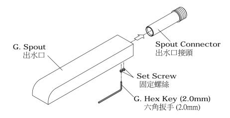
\* Loosen the Set Screws from Spout with Hex Key(2.0mm), and disassemble the Spout Connector.
