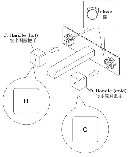
\* Turn Hot Valve and Cold Valve clockwise to closed position before install the Handle. Press both hot and cold Handles onto valve spindles until hear the click sound.
